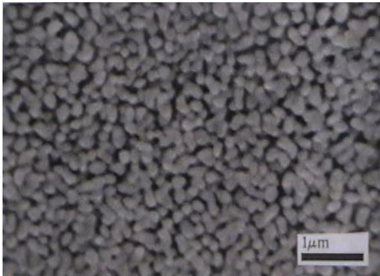
**Figure 4:** SEM micrograph showing the surface of one spherical zirconia particle shown in Figure 1, but at a higher magnification. Here the uniform individual zirconia crystallites can be seen.
