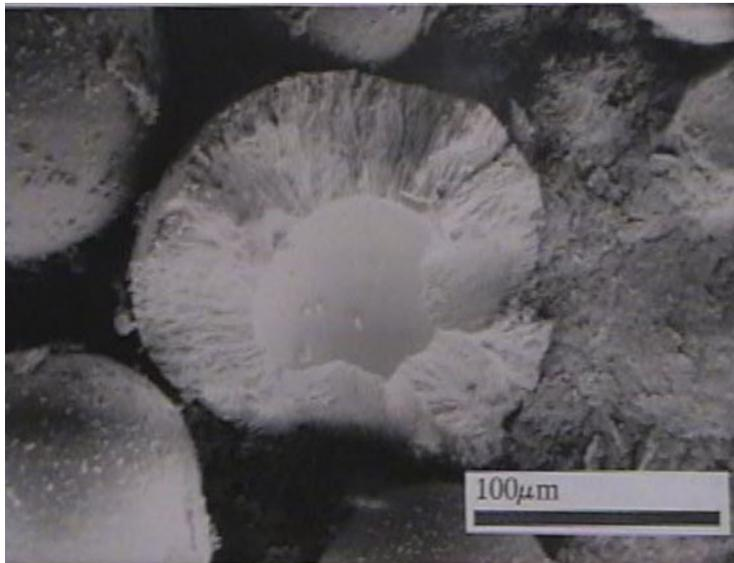
**Figure 6:** SEM micrograph showing the internal cross sectional microstructure of a cracked sphere seen in Figure 1.
