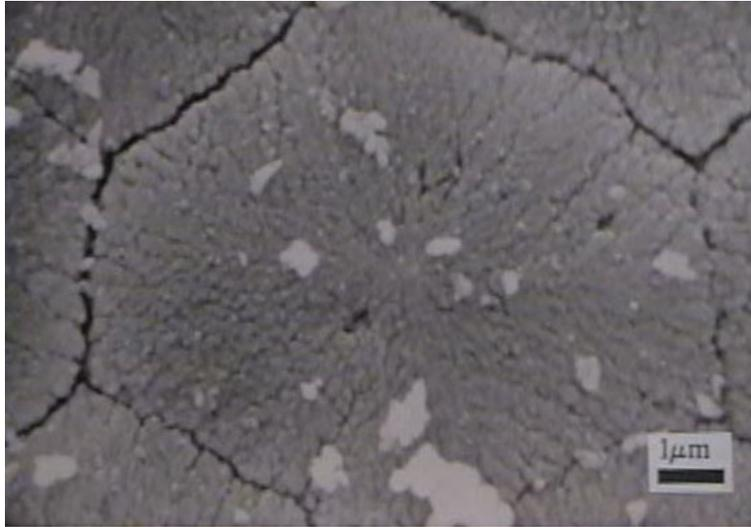
**Figure 3:** SEM micrograph showing the surface of one spherical zirconia particle shown in Figure 2, but at a higher magnification.
